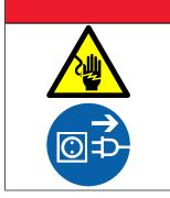
ELECTRICAL HAZARD. Cut the supply voltage to the light using the main switches before replacing the bulbs of the working and driving lights. Exercise extreme caution when performing maintenance or repair work on HID gas discharge lamps. The light components include high voltage parts. Failure to follow these procedures will result in death or serious injury!
