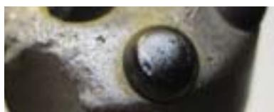
Here, the surface has become fatigued and developed microscopic cracks.
