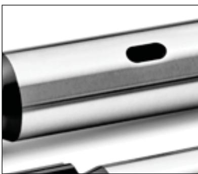
Shank adapters with external flushing can be identified by machined slots in the center of the adapter. These slots are positioned between seals inside the flushing housing/head of the rock drill.
