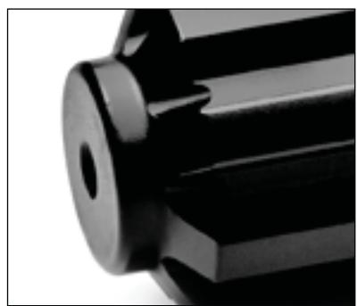
Internal flushing shank adapters use a water tube inside the rock drill. The tube fits into the end of the shank adapter and is sealed with an O-ring. This allows water to transfer from the rock drill to the shank adapter, which in turn allows it flow through the rest of the drill string.
