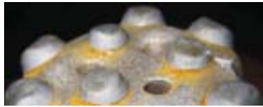
The height of the cemented carbide diminishes as wear progresses, resulting in it wearing flat.
