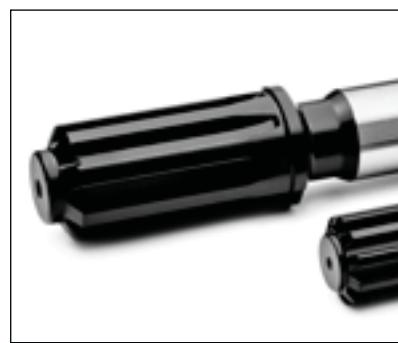
Hydraulic shanks generally have at least a 5 to 14-spline configuration. Pneumatic shanks tend to have internal or through-flushing. They can be identified by their lugs or 4-spline configuration.
