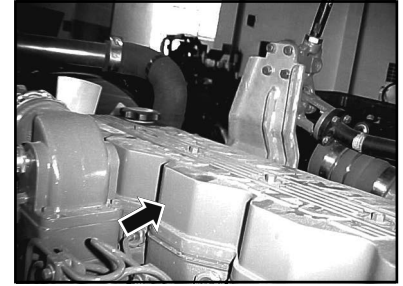
Single piece cylinder head cover (common valve cover)
