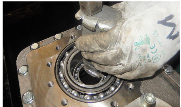
Put the assembled case with the cover into the upper part. Insert the bearing 6010 #84 into the gear ( z=25 )
