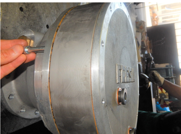
Inset the allen screws 10x1,5x100 for fixing
