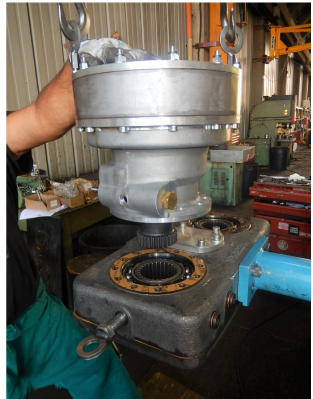
Assemble the planetary gear on the assembled case (screws 12x1,75x35 + schnorr washers)
