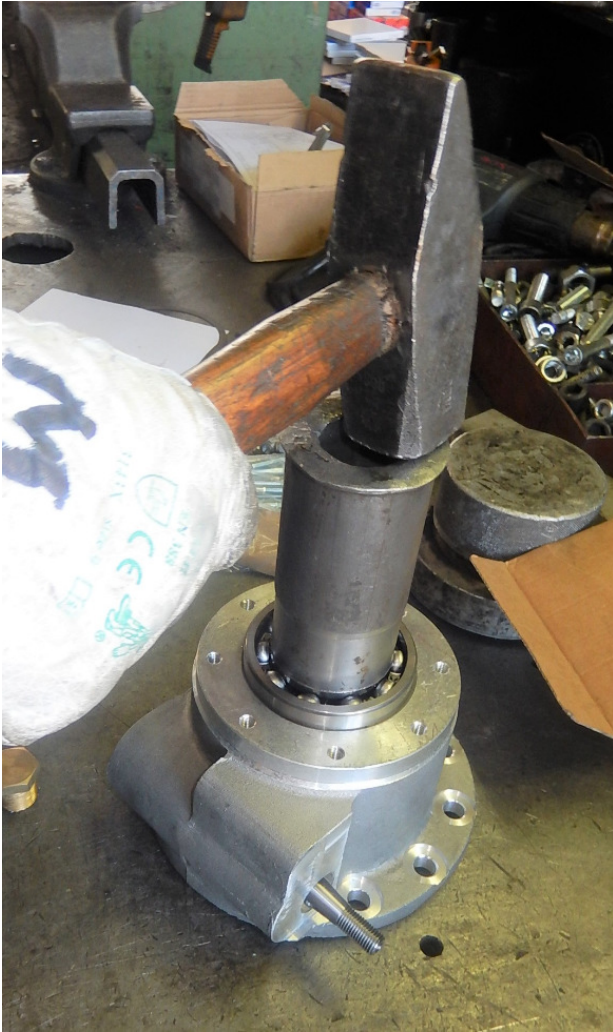
Beat slightly on the bearing by a proper punch plant the shaft and the bearing
