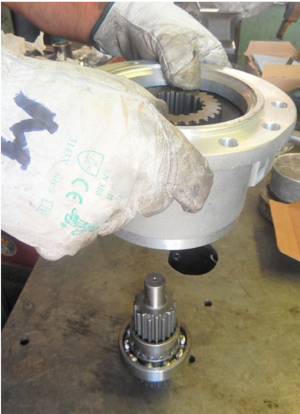
Rotate the case to slide out the shaft
