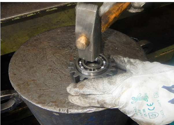
Plant the bearing 6205 into the satellites #25, slightly beat with an hammer
