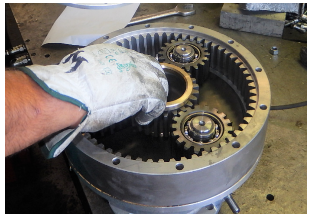
Remove the shim on the solar gear
