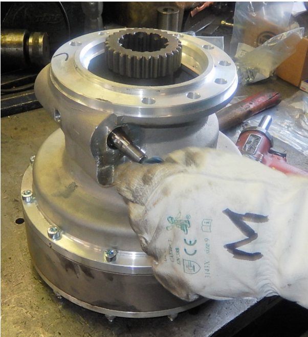
Insert the oil seal # 71 on the fork shaft
