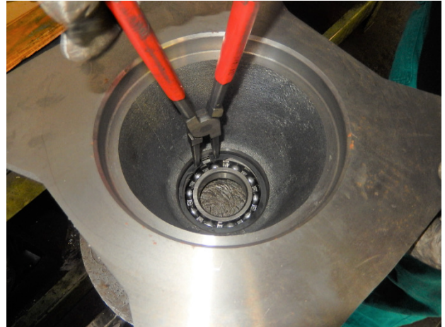
Put the support on a bench and extract the elastic ring I90 #45
