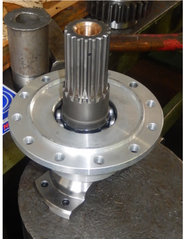
Plant the bronze bushing #66 on the shaft
