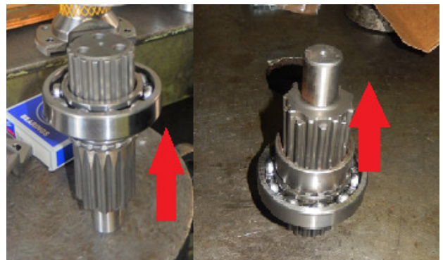
Disassemble the bearing 6210 and the spacer from the shaft
