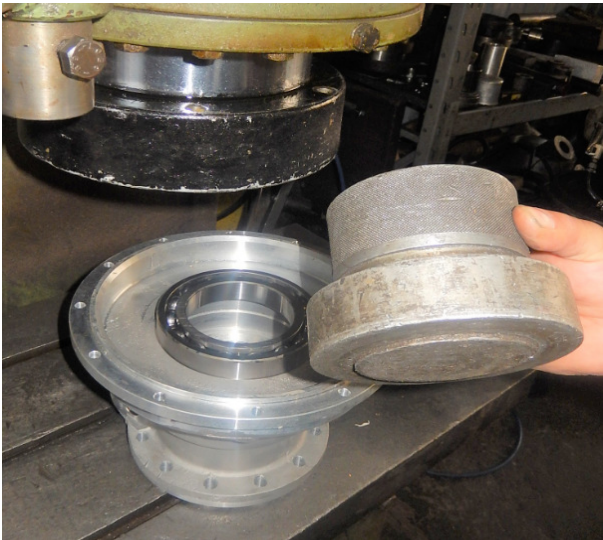
Put the case under a press and position the first bearing 6019 #7
