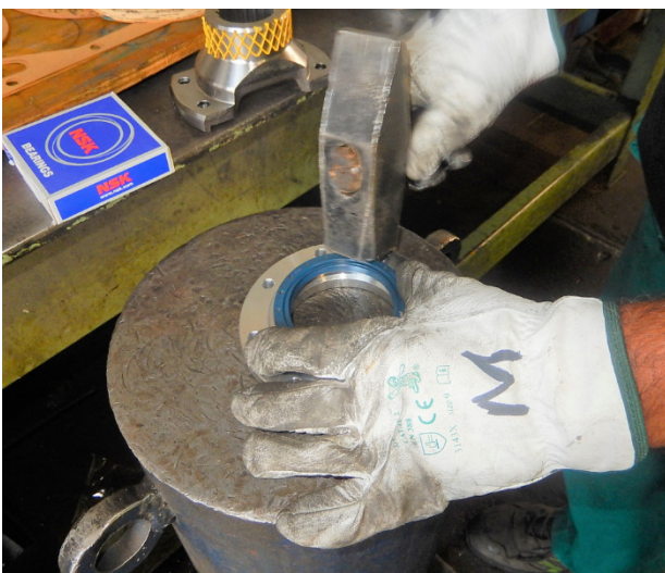
Insert the oil seal 70x90x10 #59 into the cover. Be careful not o damage it
