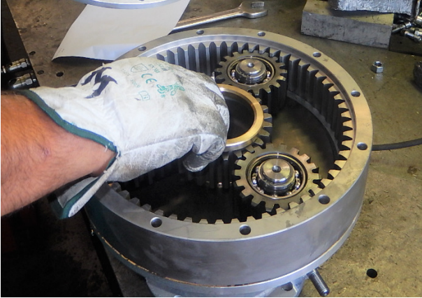
Position the shim on the solar gear
