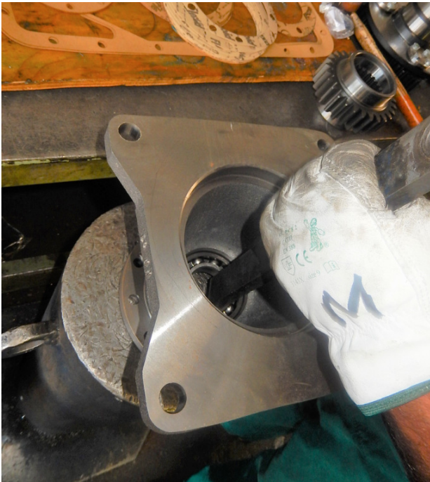
Plant the bearing 6210 into the support.
