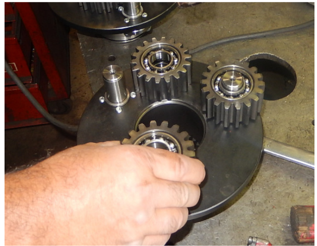
Heat the bearings with a termic gun to extract them easily
