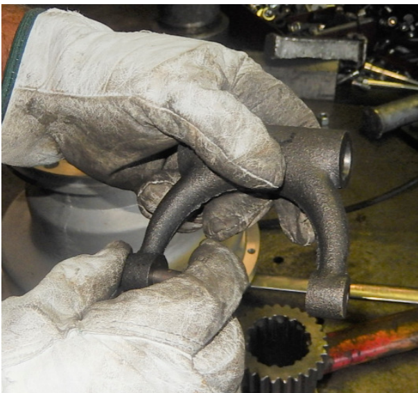
Put the sliding element #37 in the fork
