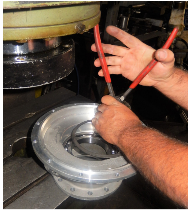
By the pliers, insert the elastic ring 1145 #18 to fix the bearing
