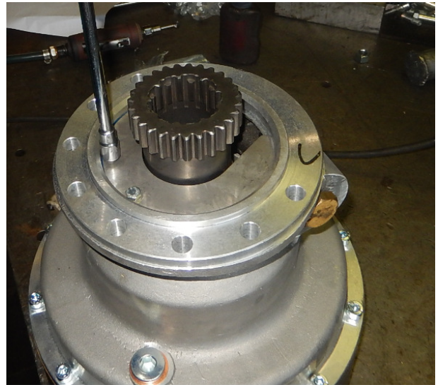
Screw the oil protection with screws 6x16 and schnorr washers d.6
