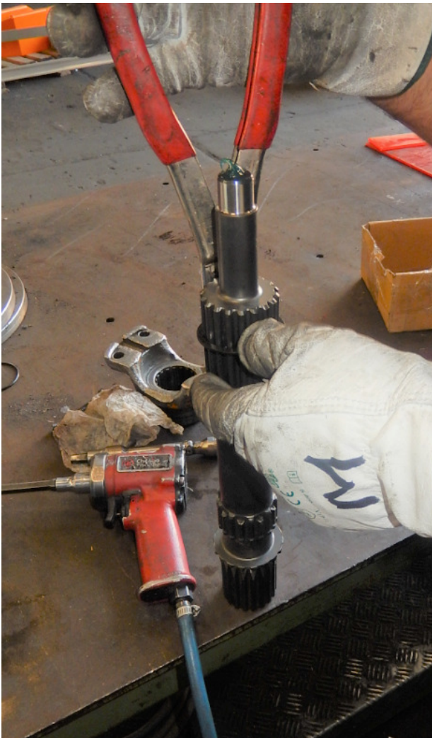
Spread some grease on the primary shaft and install the elastic E50 in its seat
