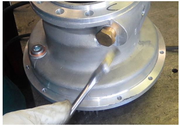
Screw the bushing plug (chck eventually the need of thickness)
