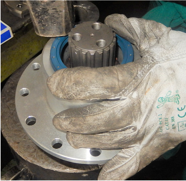
Plant the oil seal 70x90x10 #59, beat slightly not to damage it.
