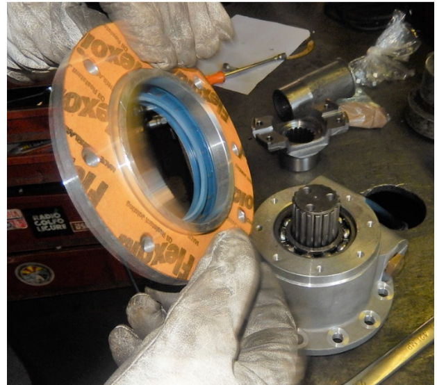
Position the paper gasket under the cover (lubricate it)
