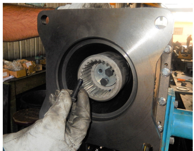
Insert the elastic ring I90 to fix the bearing (use the proper pliers)
