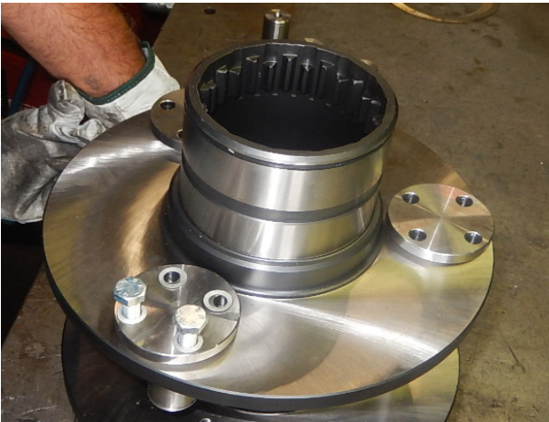
Insert the three pins #20 into the holder #19. Fix with screws d.8 and schnorr washers
