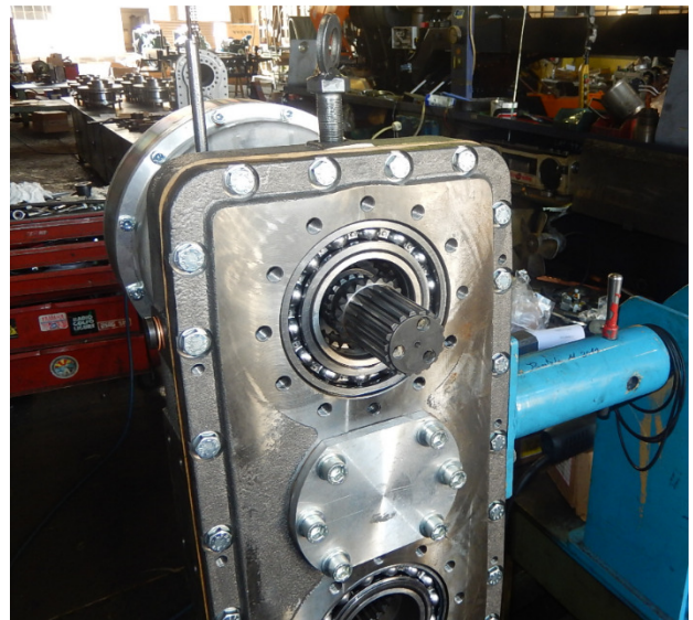
Insert the primary axle #47 into the case
