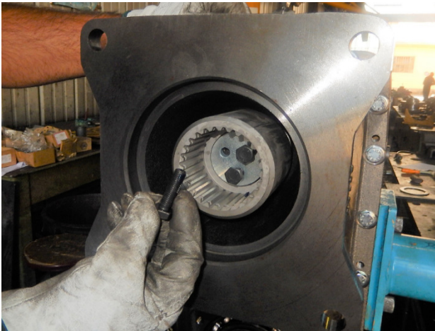
Remove the three screws fixing the external sleeve #46 to the shaft. Extract the external sleeve
