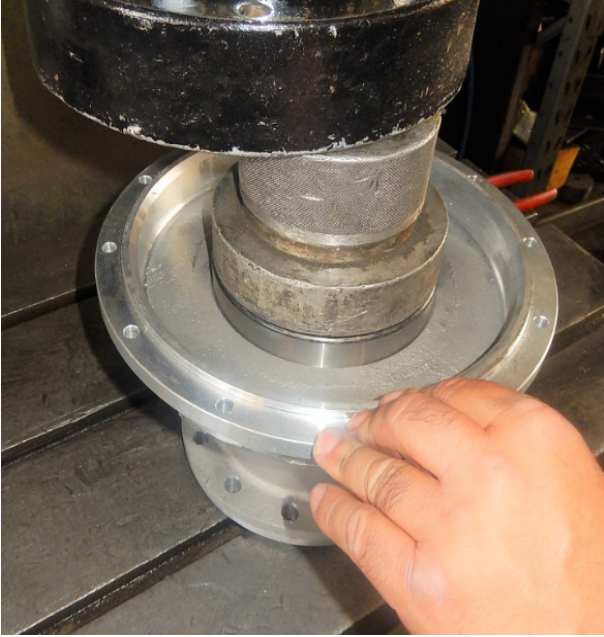
Plant the second bearing 6019.
