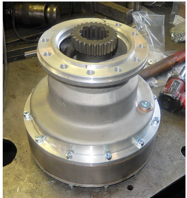
Rotate the planetary group and insert the toothed sleeve #39 into the sliding elements of the fork
