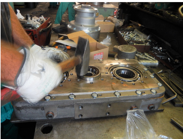
Plant the remaining bearings in the holes
