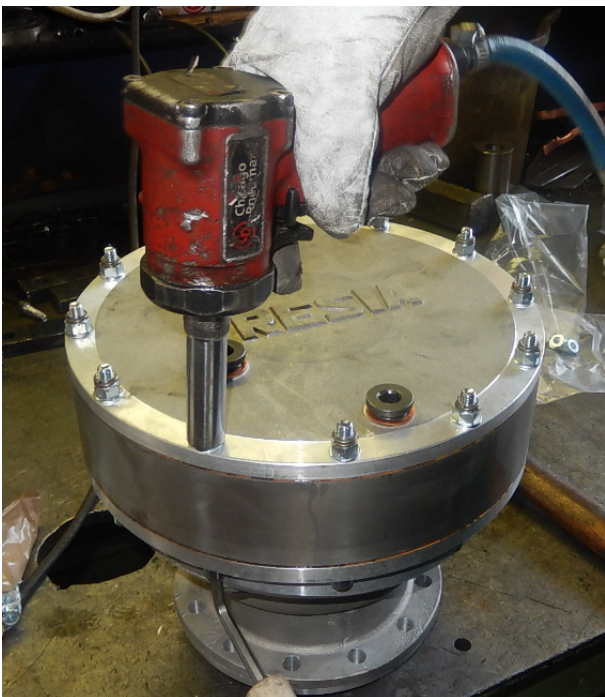
Rotate the group and unscrew the cover bolts
