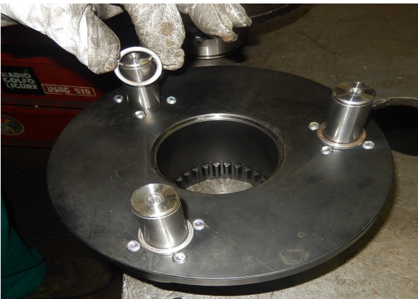
Rotate the holder case and insert the shim #23
