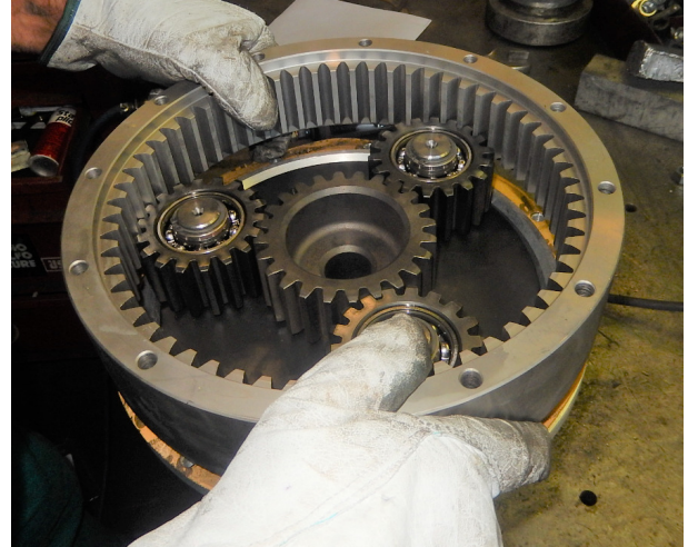
Insert the internal toothed wheel #43 on the satellites
