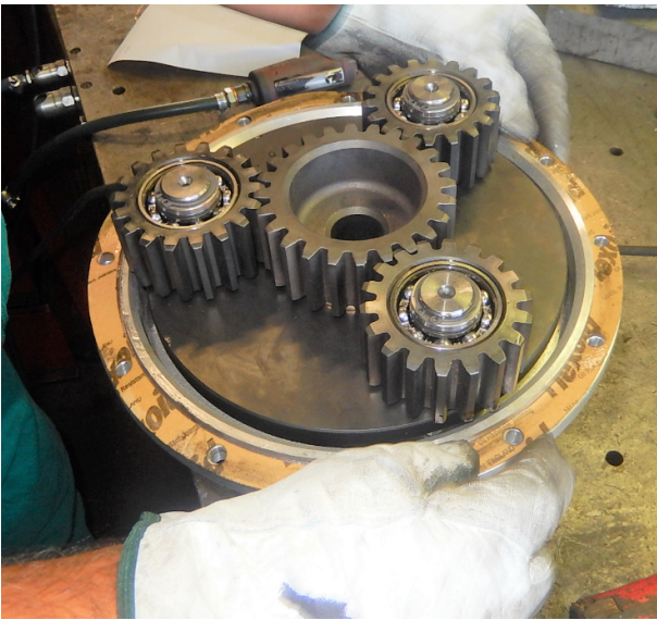
Lubricate the paper gasket and put it in the edge
