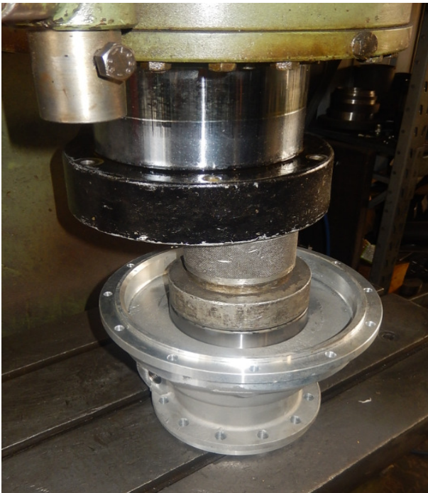
By a means of the proper beater, insert the bearing in the bottom of the case
