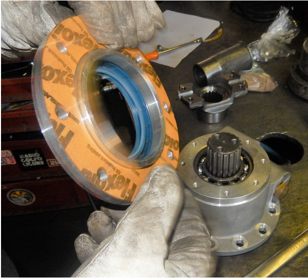
Remove the cover #63 and extract the oil seal
