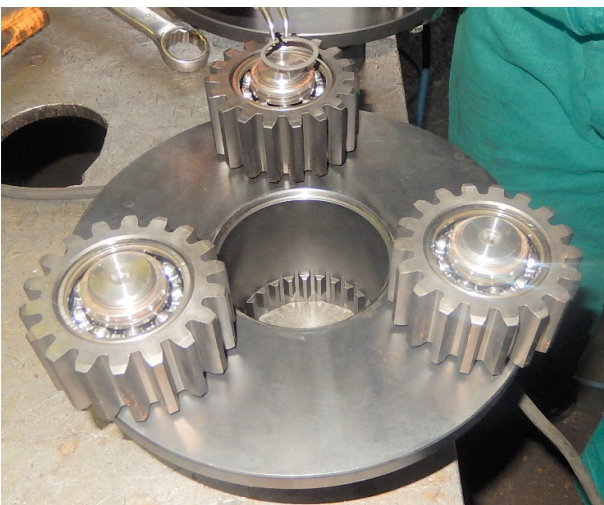
Remove the elastic rings fixing the satellites to the pins
