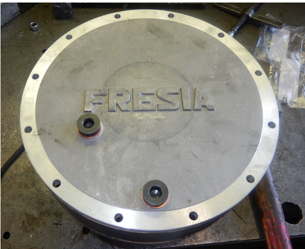
Screw the cover on the group and install the oil plugs with copper washers.
