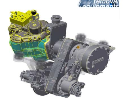
These motors are designed primarily to be combined with other products in closed circuit systems to transfer and control hydraulic power. Series H1 motors have a large maximum/minimum displacement ratio of 5:1 and high output speed capabilities.
